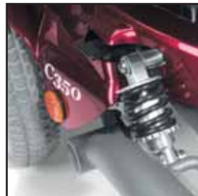
4-wheel adjustable independent suspension for comfort and grip.
