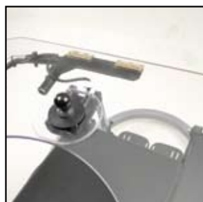
A joystick operated power wheelchair which works in a direct and predictable way.
