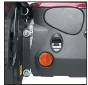
Easy access external circuit breaker switch
